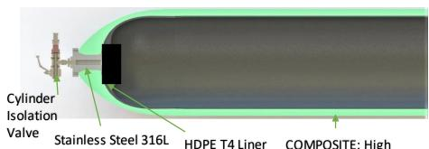
COMPOSITE: High Strength Fibre glass and Epoxy
